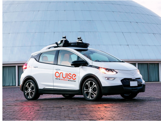
(b) Cruise autonomous prototype was recently tested in the streets of San Francisco without backup driver;
