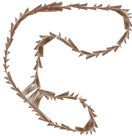
Figure 3.11: Example of the GraphSLAM sparse-graph representation. The edges connecting the nodes define the constraints with an associated error that will be minimized during the optimization process.
